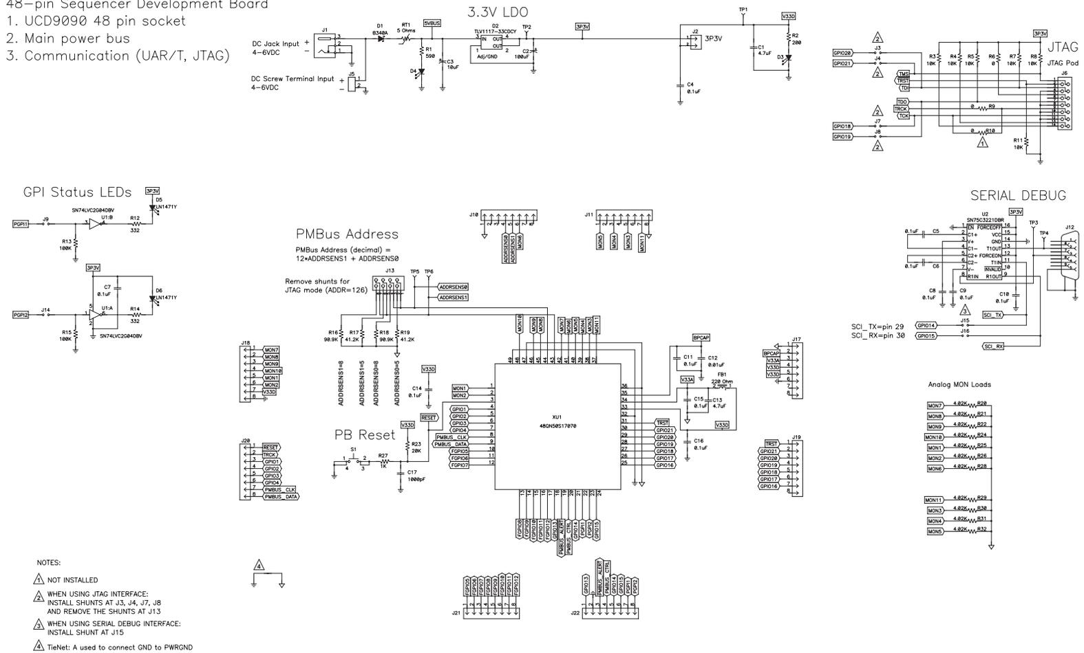
Figure 2. UCD90SEQ48EVM-560 Schematic, Sheet 1 of 2
