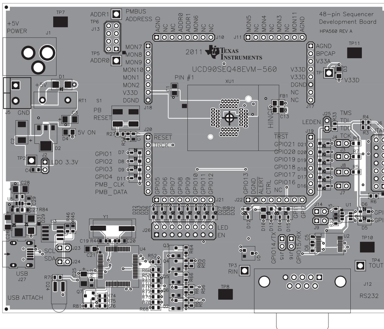
Figure 4. Top-Side Layout/Routing
