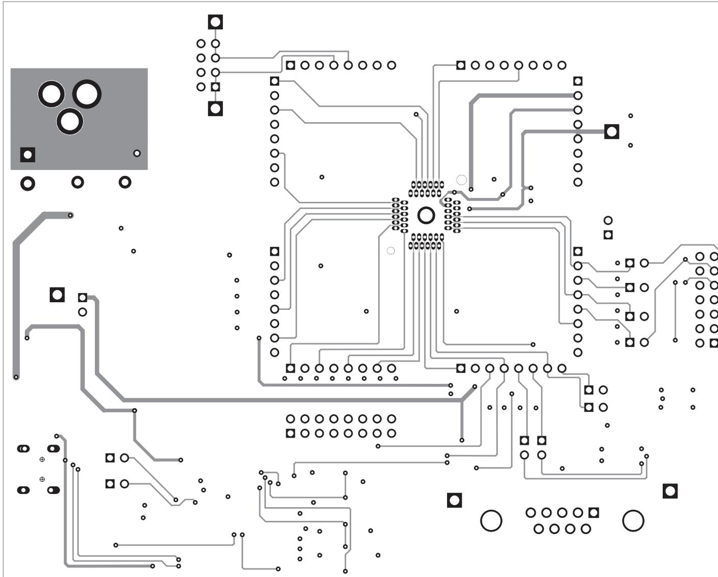
Figure 5. Layer-2 Routing
