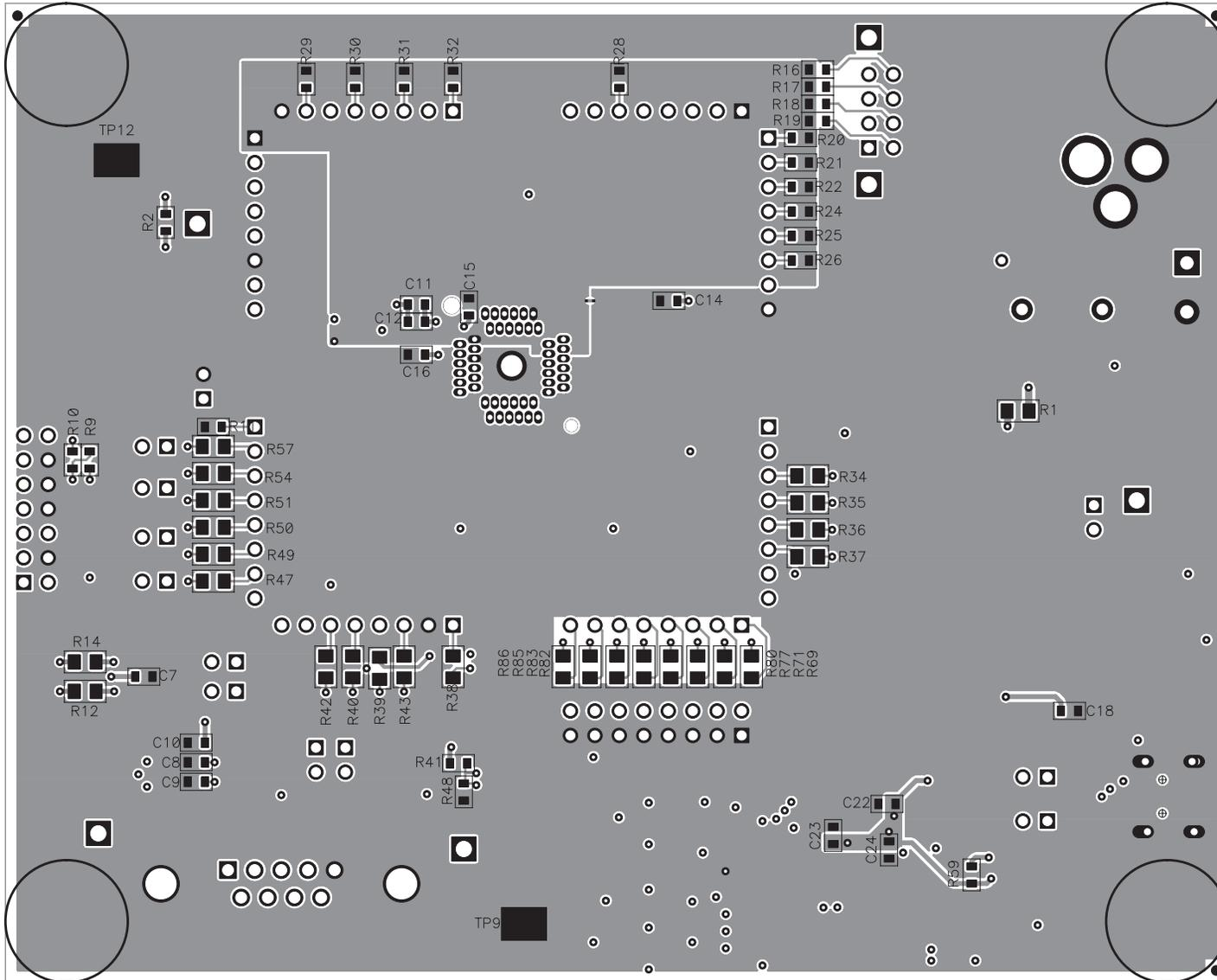
**Figure 7. Bottom-Side Placement/Routing**
