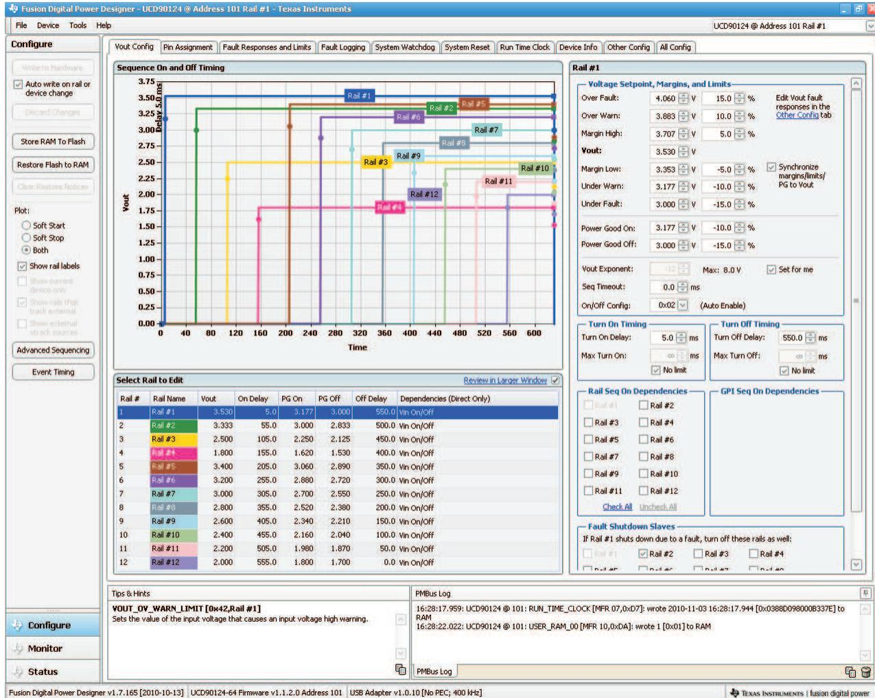
Most of the GUI control features are available from the Configure window. Monitor and Status information is available from the respective buttons on the GUI lower left. A typical Monitor window follows.
