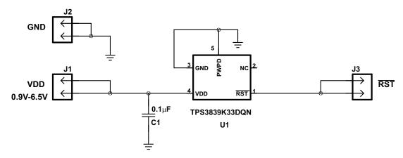
Figure 4. TPS3839K33EVM-112 Schematic
