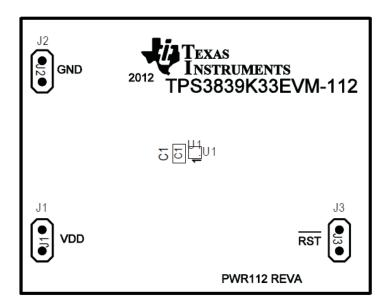
Figure 1. Assembly Layer
