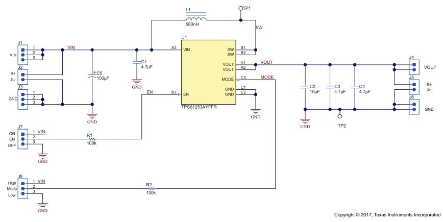
Figure 8. TPS61253AEVM-803 Schematic
