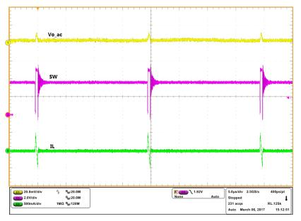
Figure 7. Output Ripple in Ultra-Sonic Mode ( $V_{IN}$  = 3.6 V, no load)
