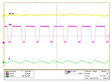
Figure 6. Output Ripple in FPWM ( $V_{IN}$  = 3.6 V,  $I_o$  = 50 mA)
