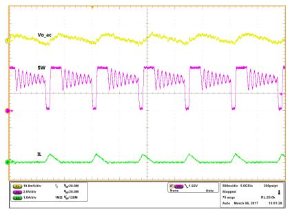
Figure 4. Output Ripple in PFM Mode ( $V_{IN} = 3.6 V$ ,  $I_0 = 50 mA$ )
