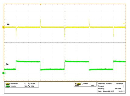
Figure 3. Load Transient ( $V_o = 3.6 V$ ,  $I_o = 0.5 A$  to 1.5 A)
