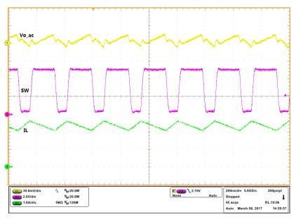
Figure 5. Output Ripple in PFM Mode (V<sub>IN</sub> = 3.6 V, I<sub>o</sub> = 1.5 A)
