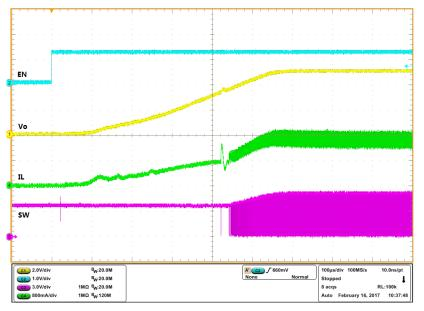
Figure 1. Startup Waveforms (R<sub>load</sub> = 5  $\Omega$ )
