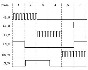
Figure 3. High-Side PWM Sequence
