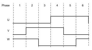
Figure 1. Hall Sensor Outputs
