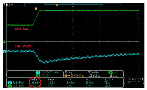
Figure 4-4. Transient Response to Load Step 9A to 18A at 1A/µs
