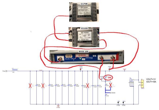
Figure 4-7. Frequency Response Test Setup
