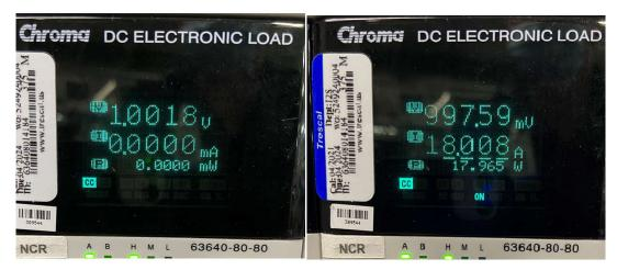
Figure 4-1. Output Voltage Regulation
