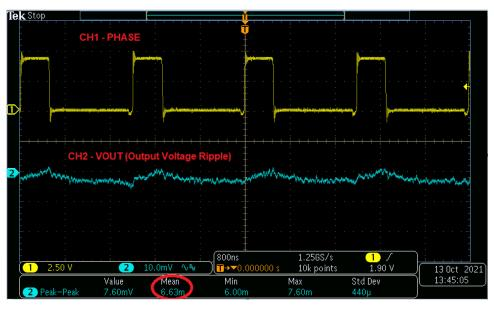
Figure 4-2. Output Voltage Ripple VIN = 5V, VOUT = 1V, IOUT = 18A
