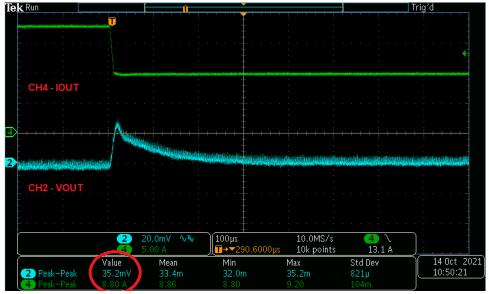
Figure 4-5. Transient Response to Load Step 18A to 9A at 1A/µs
