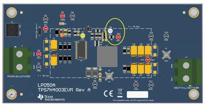
Figure 4-6. EVM Modification to Measure Frequency Response
