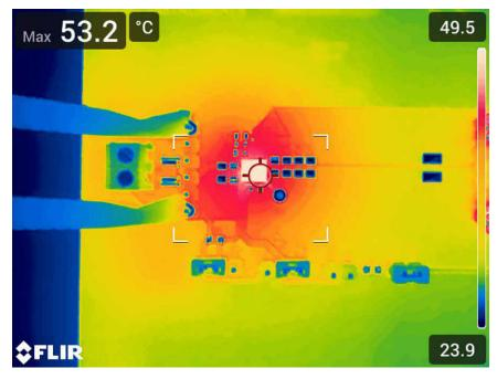
Figure 4-2. Thermal Performance (TPSM82866AA0HEVM,  $V_{IN}$  = 5 V,  $V_{OUT}$  = 1.2 V,  $I_{OUT}$  = 6 A)
