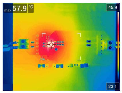
Figure 4-1. Thermal Performance (TPSM82866AA0SEVM,  $V_{IN}$  = 5 V,  $V_{OUT}$  = 1.2 V,  $I_{OUT}$  = 6 A)
