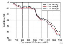
Figure 7.3 x LO Relative Gain versus Temperature
