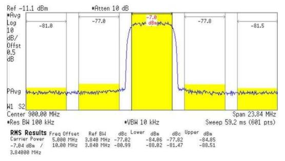
Figure 4. WCDMA Spectrum at 900-MHz LO at Zero-IF
