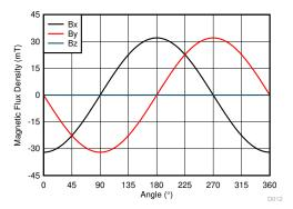
Figure 7. On-Axis Field Components
