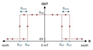
Figure 4. Omnipolar Hall-Effect Switch Functionality
