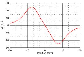
Figure 6. Magnetic Field for Linear Slide-By Magnet
