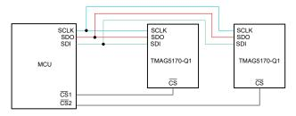
Figure 6. Simplified Block Diagram
