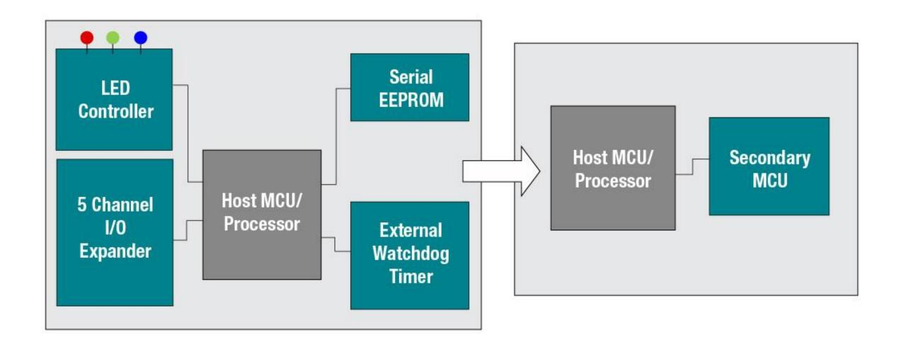
Integrate your discrete system level functions into software on your microcontroller!
