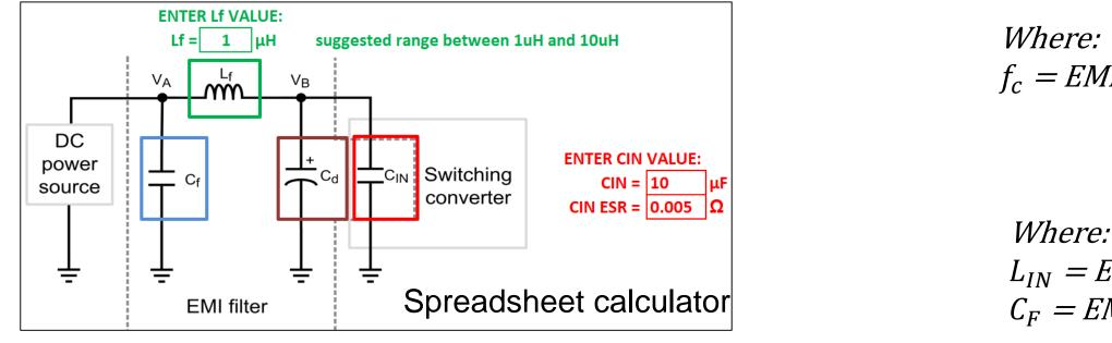
$$= 20 \log \left( \frac{\frac{I_{peak}}{\pi^2 f_{SW} C_{IN}} \sin(\pi D)}{1 \mu V} \right) - V_{MAX} \quad (1)$$
