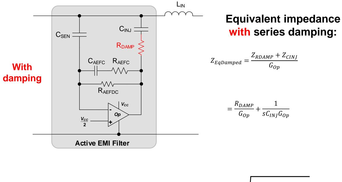
$$Q = \frac{1}{R}\sqrt{\frac{L}{C}} = 1, R = \sqrt{\frac{L}{C}} \implies \frac{R_{DAMP}}{G_{Op}} = \sqrt{\frac{L_{IN}}{C_{INJ} \cdot G_{Op}}}$$
