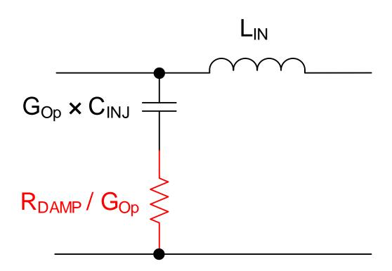
**Low-frequency** equivalent circuit with damping  $R_{DAMP} = \sqrt{$  $\left|\frac{L_{IN}\cdot G_{Op}}{C_{INI}}\right|$
