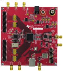
The CDCM7005 is a high-performance, low-jitter clock solution that synchronizes an onboard voltage-controlled crystal oscillator (VCXO) to a reference clock. Once the proper reference frequency and programming are applied, the CDCM7005 supplies two clock sources to the DAC and an additional three outputs for external equipment.
