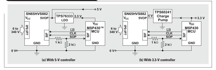
input while leaving the normal  $V_{CC}$  supply pin floating. Figure 9 shows two back-supply options for interfacing to a 3.3-V controller. In Figure 9a, the 5-V system supply powers the DIS directly but requires an LDO to supply the controller. In Figure 9b, a 3.3-V supply powers the controller directly but requires a charge pump to boost the supply voltage to the required 5-V level of the DIS.
