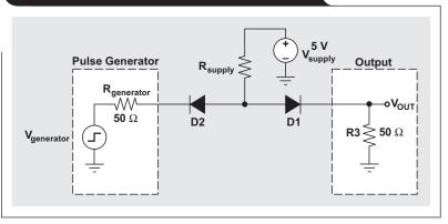
can be used to clean up the low-voltage level of the generated signal. The FBPG clamps the falling voltage to ground at the cost of a bigger overshoot. This gives test engineers some control over trade-offs in the test setup. Similarly, a flat-top pulse generator can be used to clean up the highvoltage level.
