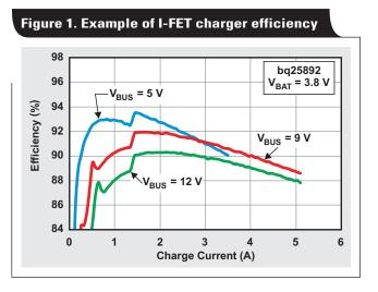
With a 9-V input adapter, a battery charger with 91% efficiency was set to provide a 3-A charging current to a 3.8-V charged battery with loses of
