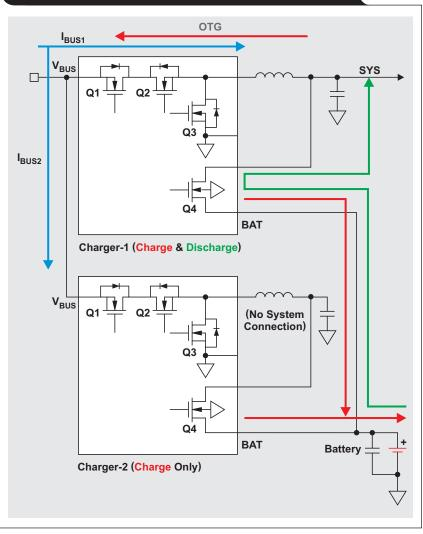
optimization (ICO) to extract maximum adapter power without causing loop instability at their mutual  $V_{BUS}$  node. Therefore, each charger's current-limit feature should be set to half the adapter's maximum output current. Inductor current ratings may also be reduced by half as well.
