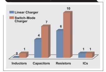
The lower BOM count in a linear charger can translate into application area savings. Any passive elements not used saves space needed for the charger. An inductor is not needed in a linear charger, which also saves space as shown in Figure 5. In low-power applications where space is critical, linear chargers can be a better fit.
