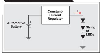
this circuit, the LED driver is directly connected to the automotive battery. Depending on the number of LEDs in the string and the amount of current being driven into the string, the constant-current regulator could be based on a linear driver circuit or a switching driver circuit.
