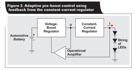
the worst-case LED string voltage and the worst-case dropout voltage of the linear constant-current regulator, which is assumed to be 1 V. This approach to choosing the linear constant-current regulator voltage guarantees startup for all conditions. Using the LED and linear LED driver parameters in Table 1, the pre-boost voltage is 29 V, as given by Equation 2.
