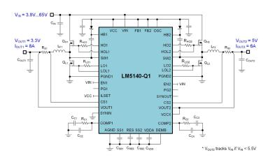
*Figure 3:* Wide  $V_{IN}$ , low  $I_Q$  dual-channel synchronous buck controller for automotive applications.
