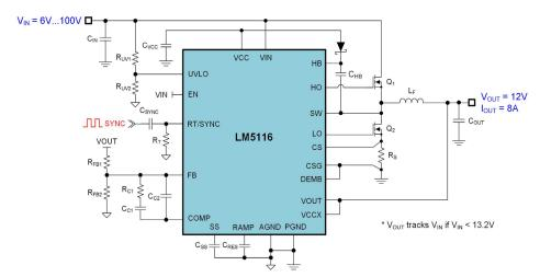
Figure 2: Robust synchronous buck converter with 6 V to 100 V input voltage range.
