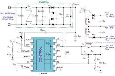
Figure 4: AC- or DC-powered Fly-Buck solution supplying ±15 V isolated rails.
