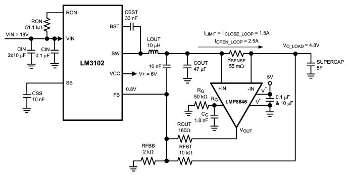
Figure 1. SuperCap Application with LM3102 Regulator and LMP8646 Precision Current Limiter
