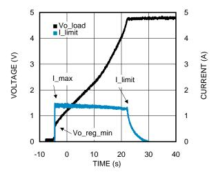
Figure 3. SuperCap Application with LM3102 Regulator Plot
