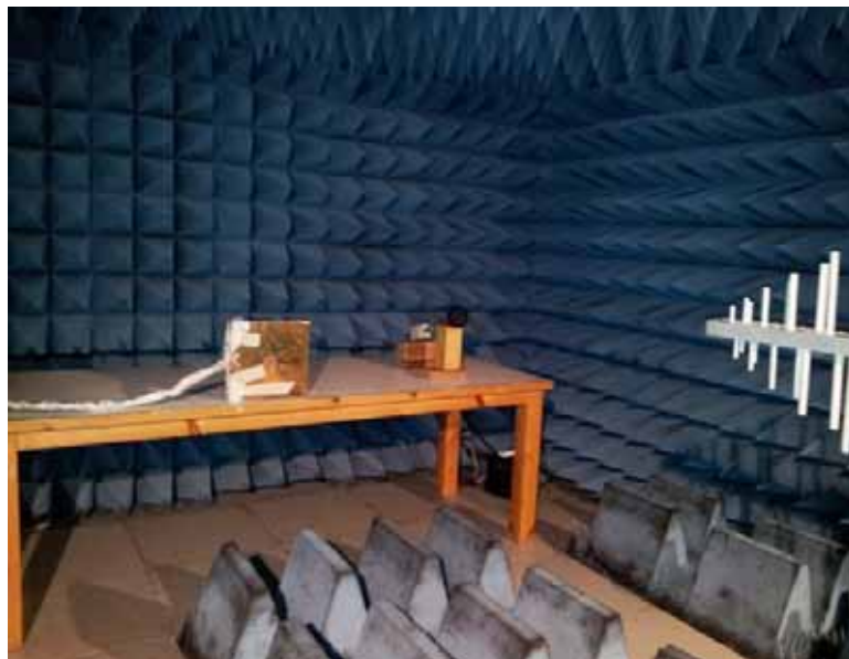
Photograph 8.1.4 Setup for radiated immunity to RF electromagnetic field test, general view, radiation from EUT pins
