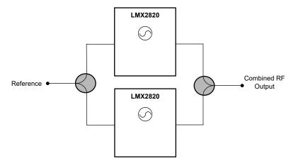
Figure 2-1. Combined LMX2820 Block Diagram
