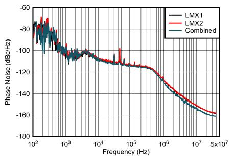
Figure 2-2. Combined LMX2820 Phase Noise Performance
