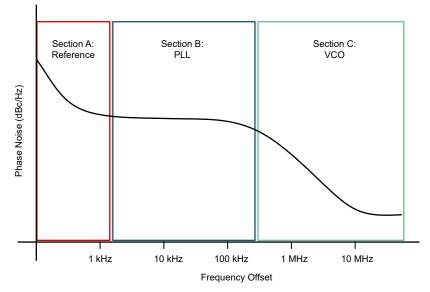
Figure 1-1. Phase Noise Breakdown by Section
