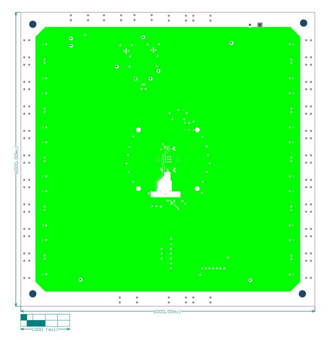
Figure 9. Internal Power Plane, Layer #3 (Not to scale)
