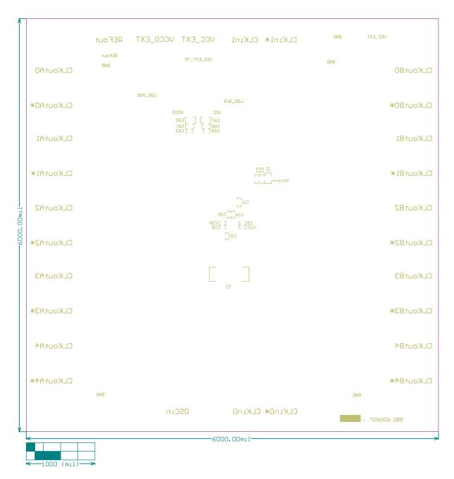
Figure 12. Bottom Silkscreen (Top view, Not to scale)
