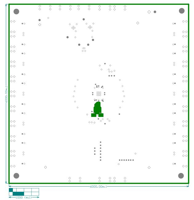
Figure 8. Internal Ground Plane, Layer #2 (Layer Inverted, Not to scale)
