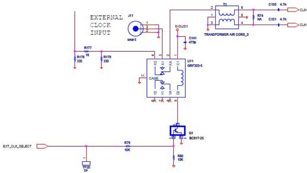
**Figure 15. External / internal clock selection circuit on ADC08D1520RB**
