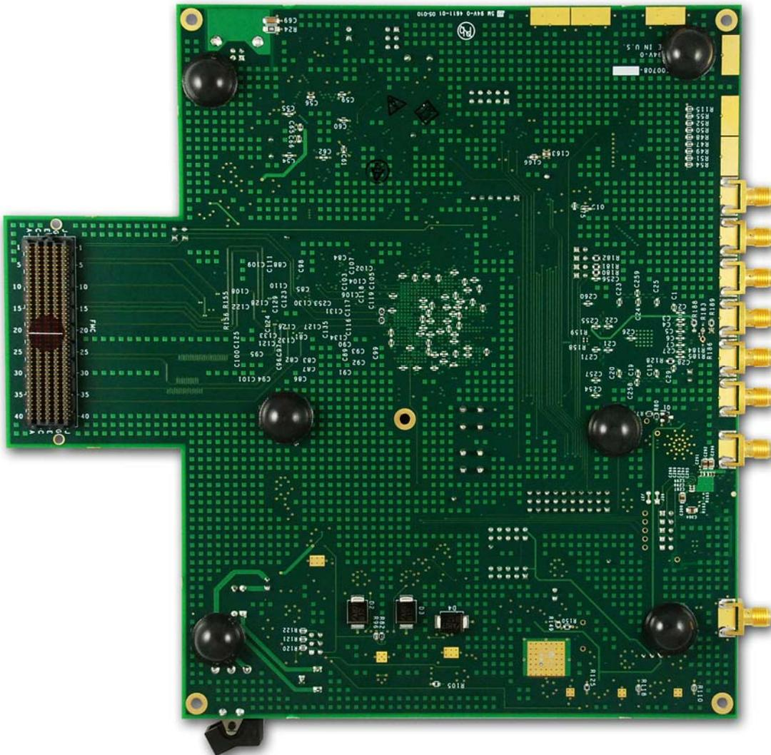
Figure 19: Bottom of ADC08D1520RB showing FMC port
