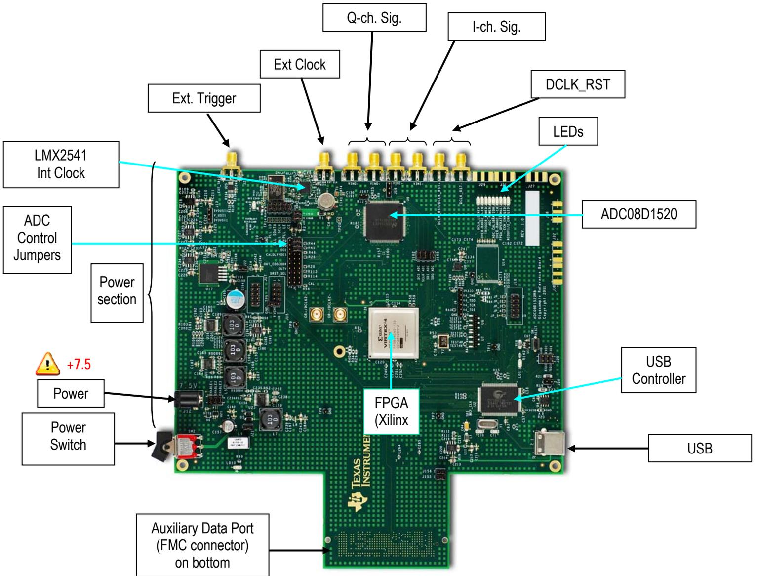
Figure 1: ADC08D1520RB Board Layout
