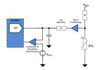
Figure 4. Example Discrete Implementation of a Temperature Monitor and Switch
