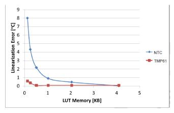
Figure 2. LUT Comparison Between PTC vs NTC
