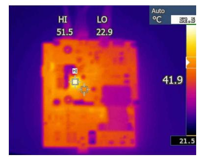
Figure 2-1. Thermal Capture of AWR2243BOOST Under Moderate Load
