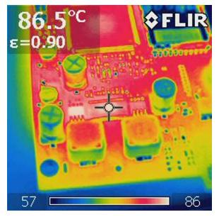
Figure 3-7. Thermal Capture of Emitted Thermal Radiation Above and IC
