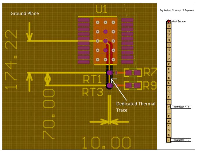
Figure 3-9. Differential Temperature Measurement Layout With Dedicated Thermal Trace and Concept of Squares Diagram
