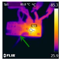
Figure 3-4. Thermal Flow Across TIDA-00982 Ground Plane
