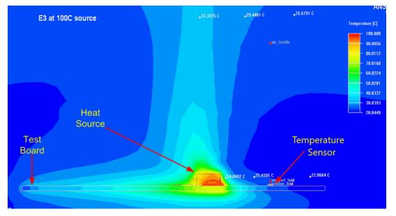
Figure 2-2. Thermal Simulation of Temperature Sensor Near 100°C Heat Source
