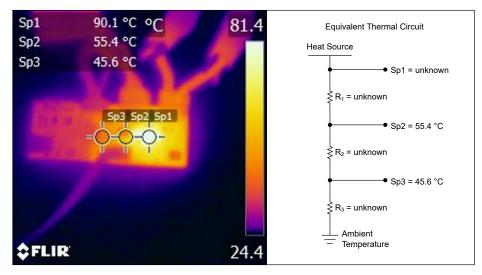
Figure 3-6. Thermal Capture of TIDA-00982 Under Heavy Load With Three Reference Points
