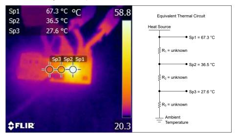
Figure 3-5. Thermal Capture of TIDA-00982 Under Moderate Load With Three Reference Points
