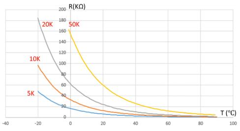
Figure 2-1. Diagram of NTC R-T Relationship With Different Resistance Values Slow response time
