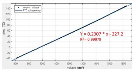
Figure 3-5. The Output Relationship Diagram of Temperature and Voltage of TMP61
