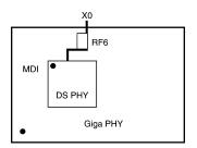
Figure 1. Use RF6 for Reduce Stubb
