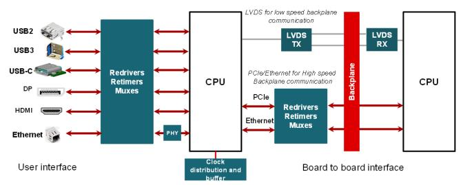
Figure 2-2. High speed interfaces inside an industrial PC system
