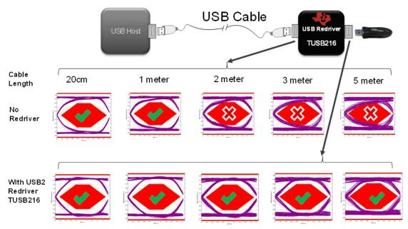
Figure 2-3. Using USB2 Redriver to Pass Compliance
