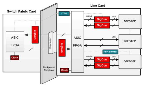
Figure 2-7. 10GbE Communication Switch using Ethernet Retimer
