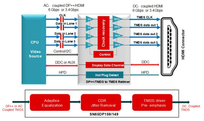
Figure 2-5. HDMI2.0 Retimer Example Using TI SN65DP159
