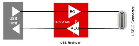
Figure 2-4. USB3 and Type-C Redriver with Adaptive EQ
