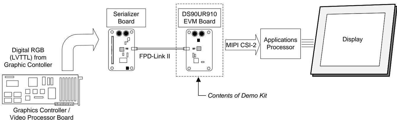
**Figure 4. Typical Test Setup for Video Application**
