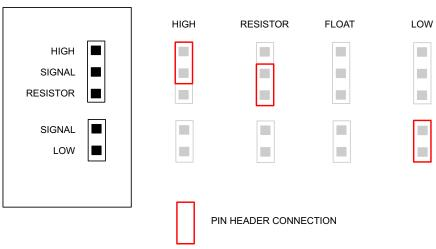
Figure 2. 4-Level IO Control on EVK
