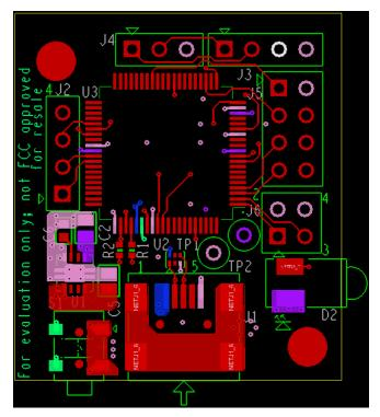
Figure 9. DPS-DONGLE-EVM Top Layer.
