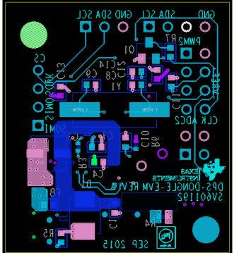
Figure 10. DPS-DONGLE-EVM Bottom Layer.
