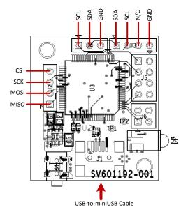
Figure 4. DPS-DONGLE-EVM Connection Diagram.
