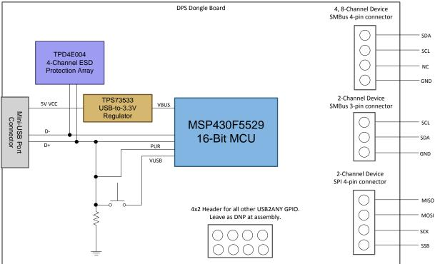
Figure 3. Simplified Board Block Diagram.
