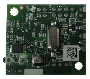
Figure 2. DPS-DONGLE-EVM Board (Back).
