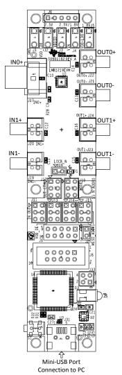
Figure 2. LMH1219EVM Input and Output Pins
