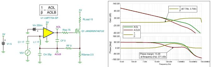
• The simple fix to this is to create a high frequency pole in 1/ $\beta$  and bypass the MOSFET at higher frequencies. By adding the capacitor CF, the amplifier returns to unity gain over the frequency range of interest. Calculate the value of CF by looking at the location of the 1/ $\beta$  zero ( $f_{z1/\beta}$ ), shown in the previous figure as 67.78kHz. The value of CF is then calculated as:
