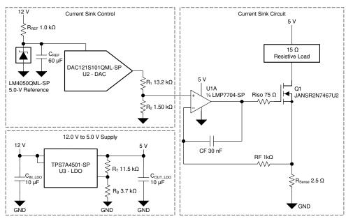
Space-Grade, 100-krad, Voltage-Controlled Current Sink (0–200 mA) Circuit
