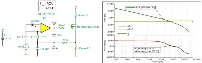
The AC simulation can be verified by the small signal step transient response. The small signal transient step response shows that the circuit has a long settling time with excessive ringing. Therefore, it is highly susceptible to oscillations.
