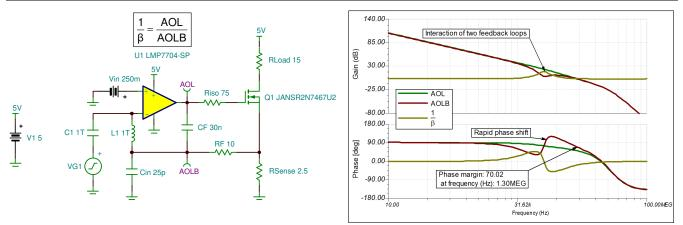
• This may be confirmed by looking at the small signal transient step response which shows oscillation at the resonant frequency of about 170kHz for small values of RF.
