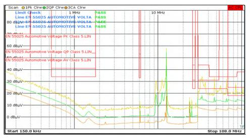
Figure 2-13. Conducted Test With 12.6-MHz Sensor Coil
