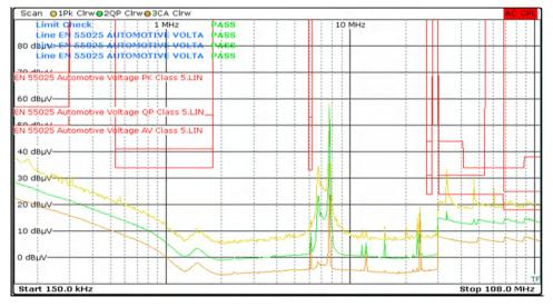
Figure 2-12. Conducted Test With 7-MHz Sensor Coil
