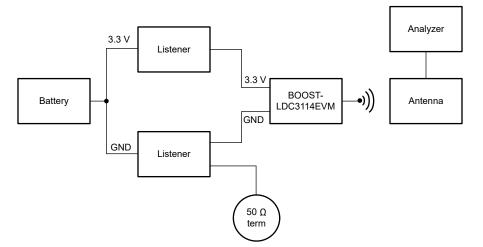
Figure 2-1. Radiated Test Block Diagram
