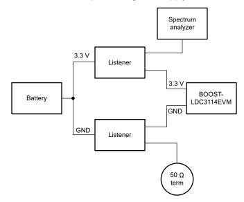
Figure 2-10. Conducted Test Block Diagram
