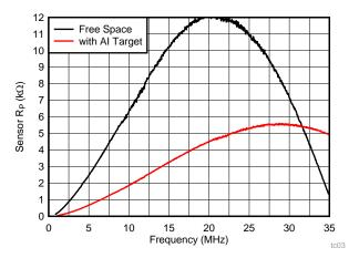
Figure 6. Coil C: R<sub>P</sub> vs. Frequency
