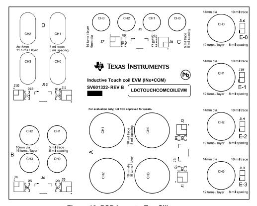
Figure 12. PCB Layout - Top Silkscreen
