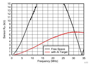
Figure 10. Coil E: R<sub>P</sub> vs. Frequency
