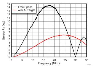
Figure 4. Coil B: R<sub>P</sub> vs. Frequency
