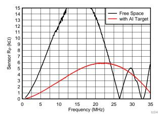
Figure 8. Coil D: R<sub>P</sub> vs. Frequency
