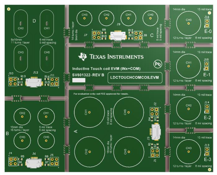
Figure 1. LDC Reference Coils Board (Top View)
