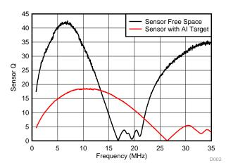
Figure 3. Coil A: Q vs. Frequency
