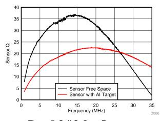
Figure 7. Coil C: Q vs. Frequency
