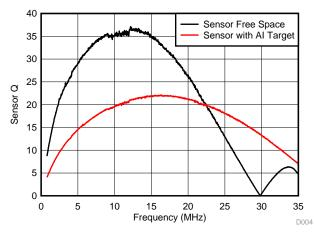
Figure 5. Coil B: Q vs. Frequency
