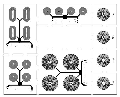
Figure 14. PCB Layout - Bottom Layer
