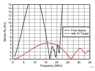
Figure 2. Coil A: R<sub>P</sub> vs. Frequency
