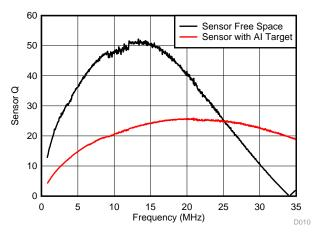
Figure 11. Coil E: Q vs. Frequency
