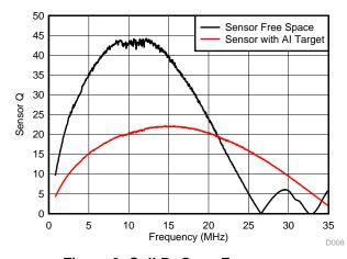
Figure 9. Coil D: Q vs. Frequency
