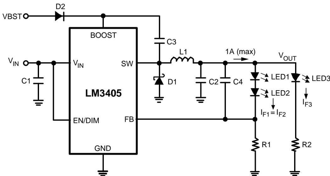
Figure 6. Driving Multiple LED Strings
