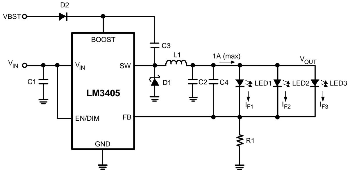
Figure 7. Driving Multiple LEDs in Parallel
