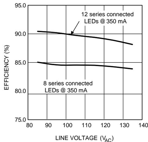
**Figure 4. LM3445 Efficiency vs Input Voltage
