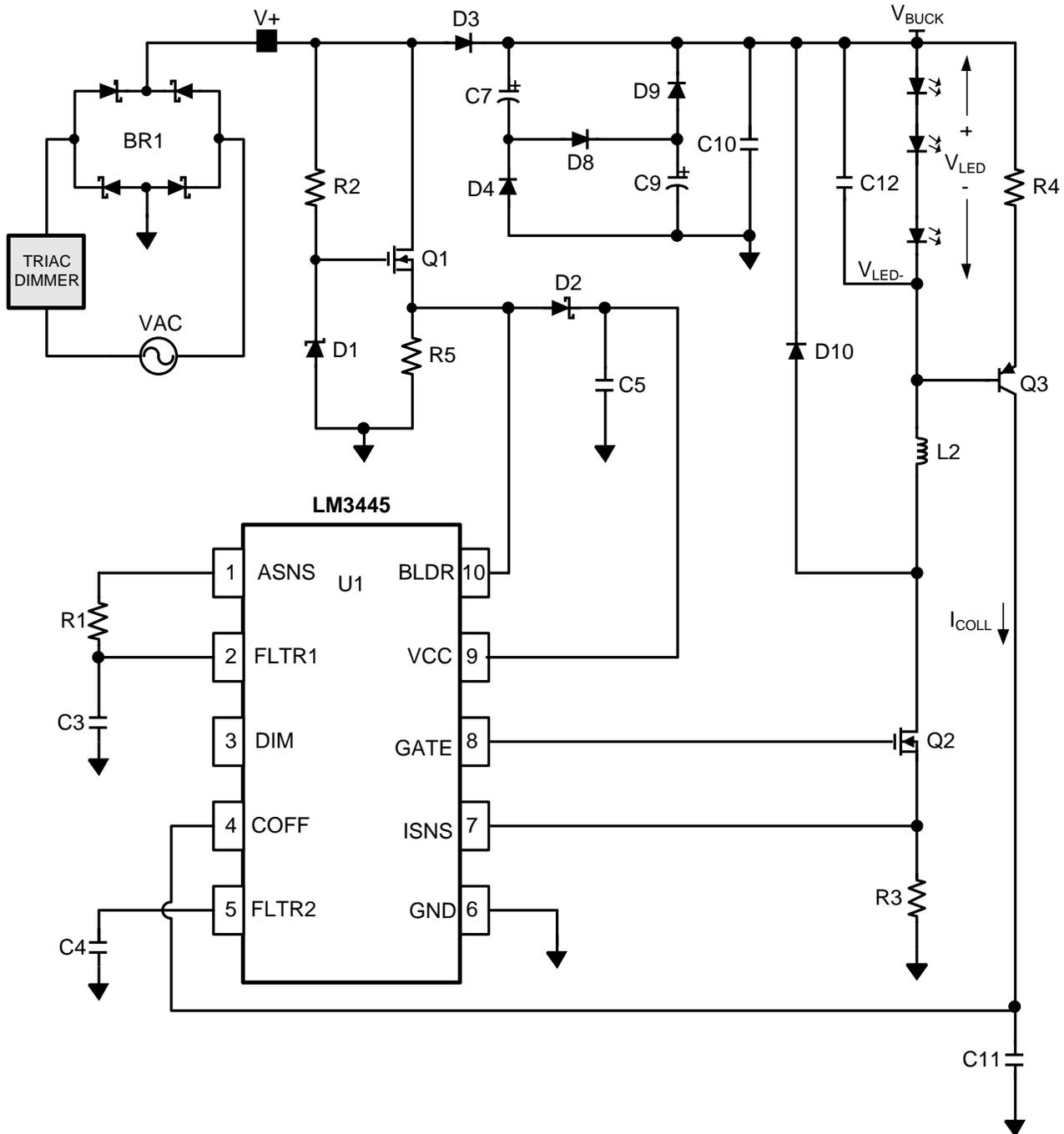
Figure 1. Simplified LM3445 Schematic
