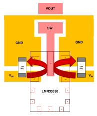
Figure 2. Demonstrating the HotRod Package Design of the LMR33630
