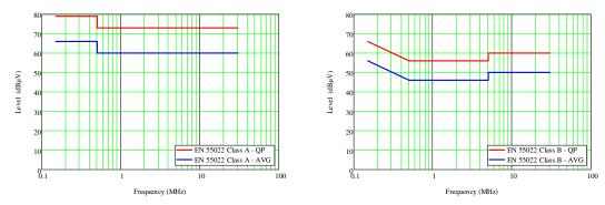
Figure 1. CISPR-22 Conducted EMI standards
