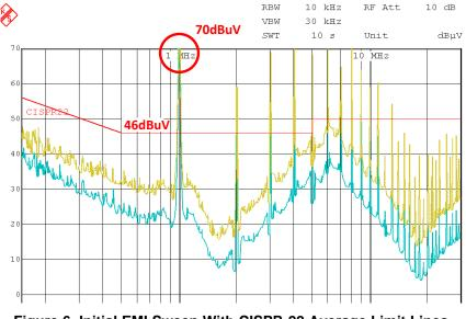
Figure 6. Initial EMI Sweep With CISPR-22 Average Limit Lines
