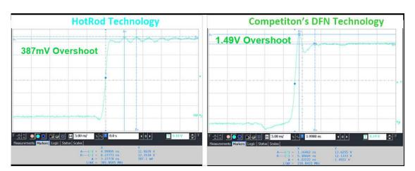
Figure 5. Illustrating Benefit of HotRod Technology for Switch Node Performance (Less Ringing)
