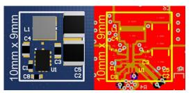
Figure 3. Illustrating Example Hotrod Layout
