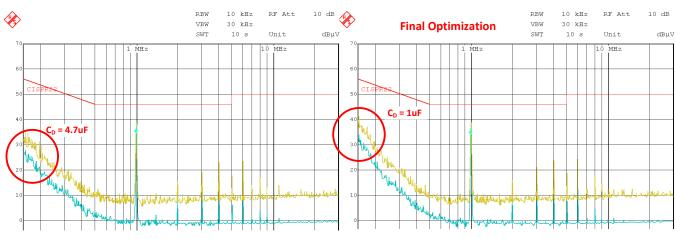
Figure 13. Damping Capacitor Filtering Comparison and Final Optimization
