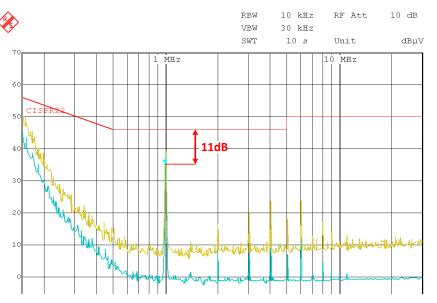
Figure 8. Passing CISPR-22 EMI Limits With a Simple LC Filter
