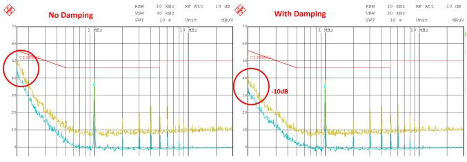
Figure 11. Comparing EMI Sweep Results With and Without a Damping Filter
