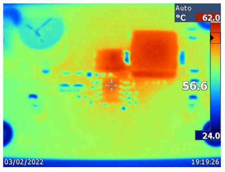
Figure 2-4. Thermal Rise on LM5013-Q1EVM (21.6cm<sup>2</sup>, 4-layer board)
