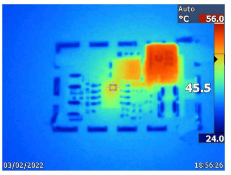
Figure 2-6. Thermal Rise on Experimental LM5013 PCB (110cm<sup>2</sup>, 4-Layer Board)
