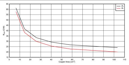
Figure 2-3. LM5013 R<sub>OJA</sub> vs. Copper Area
