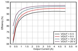
Figure 5-2. Efficiency Measurement for  $V_{IN}$  = 28-V
