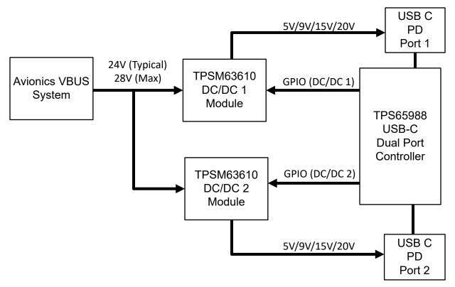
Figure 2-1. Dual-Port USB Type-C Power/Data Source
