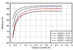
Figure 5-1. Efficiency Measurement for  $V_{IN}$  = 24-V
