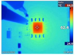
Figure 5-3. Thermal Measurement for V<sub>OUT</sub> = 5-V
