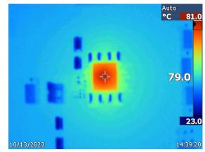
Figure 5-6. Thermal Measurement for V<sub>OUT</sub> = 20-V
