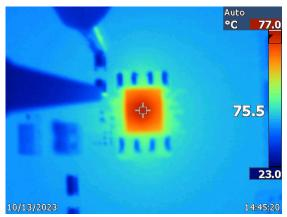
Figure 5-5. Thermal Measurement for V<sub>OUT</sub> = 15-V
