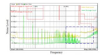
Figure 3-4. Conducted EMI Test Result With Ferrite Bead
