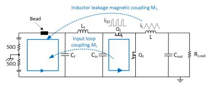
Figure 3-2. Effect of Bead Adding in Front of EMI Filter
