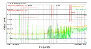
Figure 3-3. Conducted EMI Test Result Without Ferrite Bead
