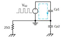
Figure 3-16. CM Noise Emission Model of Shield Added
