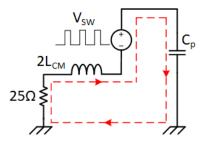
Figure 2-6. Emission Model of CM Noise
