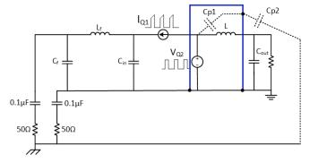
Figure 3-15. The Shield Effect on Parasitic Capacitance
