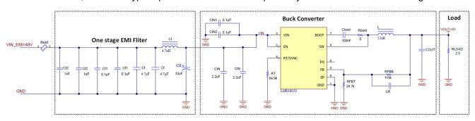
Figure 3-1. Buck Converter Schematic with EMI Filter and Bead
