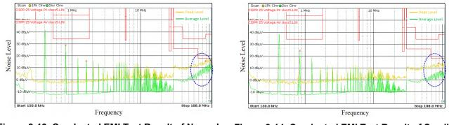
Figure 3-13. Conducted EMI Test Result of Normal Inductor
