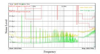
Figure 3-18. Conducted EMI Result Without Spread Spectrum
