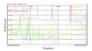
Figure 3-19. Conducted EMI Result With Spread Spectrum
