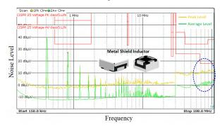
Figure 3-17. Conducted EMI Result of Metal Shield Inductor
