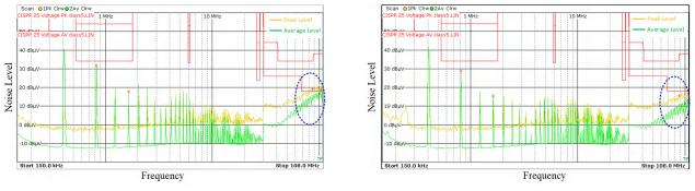
Figure 3-7. Conducted EMI Test Result of Nonsymmetrical Cin Placement
