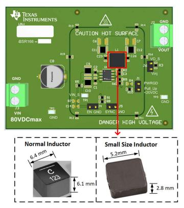
Figure 3-12. Different Size of Inductor Selection in Buck Converter
