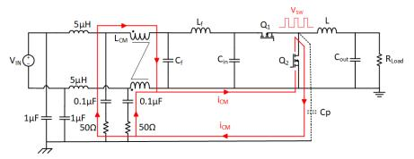
Figure 2-5. Propagation Path of CM Noise
