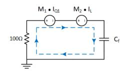
Figure 2-4. Emission Model of DM Noise Induced by Magnetic Coupling
