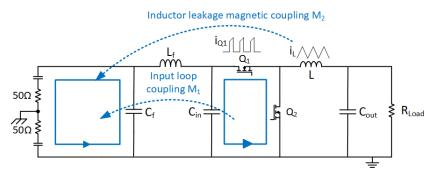
Figure 2-3. Propagation Path of DM Noise Induced by Magnetic Coupling
