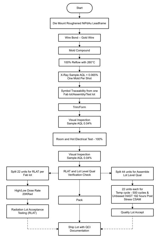
Figure 2-1. TPS7H4010-SEP Space Enhanced Plastic Production Flow Chart
