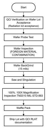
Figure 2-2. TPS7H4010-SEP Space Enhanced KGD Production Flow Chart
