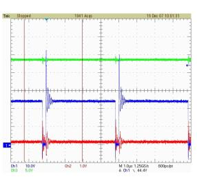
FIGURE 22, Typical protection after short circuit of the 3.3V
