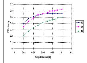
FIGURE 13, Efficiency of the complete board including the input filter at Vin=10V,24V,40V
