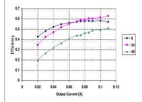
FIGURE 14, Efficiency of the complete board without the input filter at Vin=9V,24V,40V
