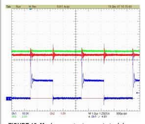
FIGURE 12. Maximum output current at minimum input voltage
