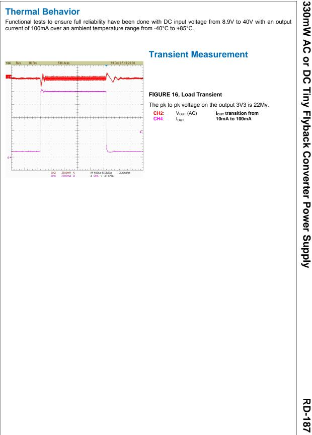
330mW AC or DC Tiny Flyback Converter Power Supply
