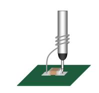
**FIGURE 6. Short Probe Connection**
