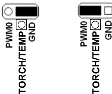
Figure 4. TORCH/TEMP Jumper Settings
