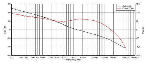
Figure 5-17. Control Loop Response,  $V_{IN}$  = 9V,  $I_{OUT}$  = 1.2A
