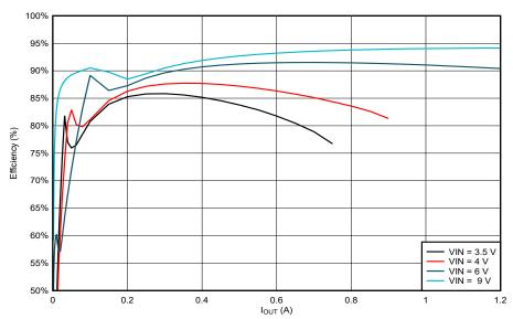
Figure 5-1. Efficiency vs Load
