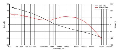
Figure 5-16. Control Loop Response,  $V_{IN}$  = 6V,  $I_{OUT}$  = 0.6A
