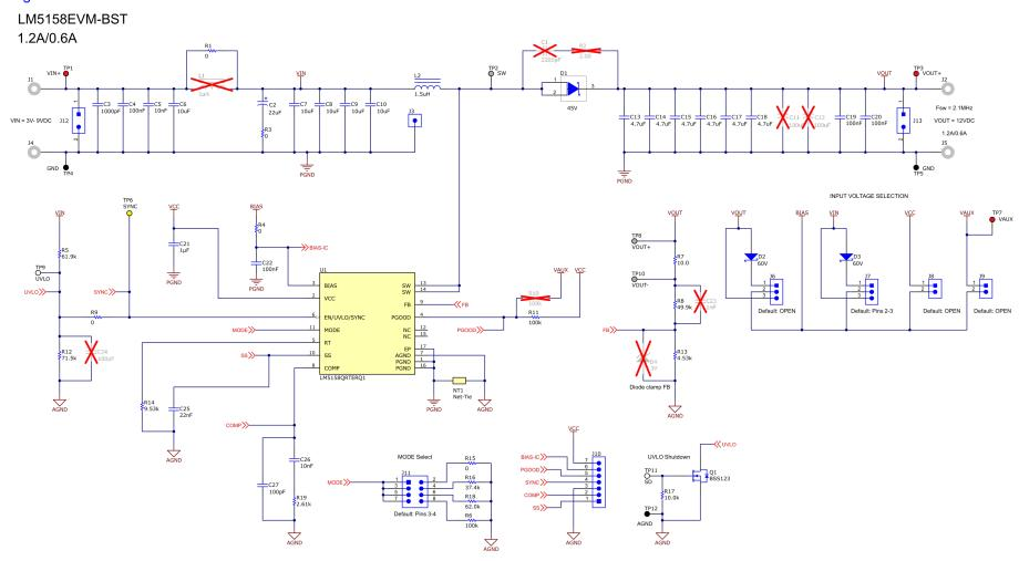
Figure 6-7. LM5158EVM-BST Schematic
