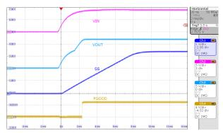
Figure 5-11. Start-Up,  $V_{IN}$  = 9V,  $I_{OUT}$  = 1.2A
