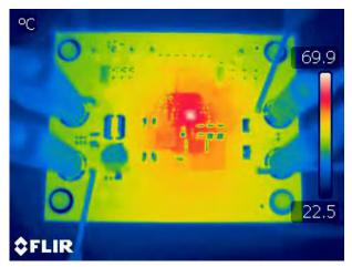
Figure 5-3. Thermal Image:  $V_{IN}$  = 3.V,  $I_{OUT}$  = 0.6A,  $V_{BIAS}$  = 3.3V, No Forced Air Cooling
