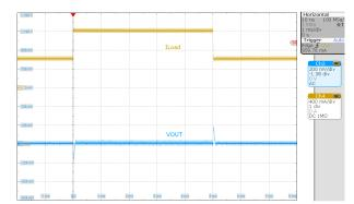
Figure 5-14. Load Transient,  $V_{IN}$  = 9V,  $I_{OUT}$  = 0.6A to 1.2A
