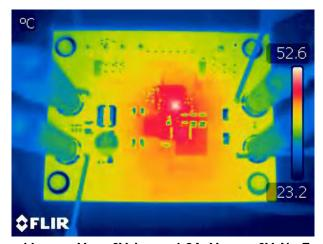
Figure 5-5. Thermal Image:  $V_{IN}$  = 6V,  $I_{OUT}$  = 1.2A,  $V_{BIAS}$  = 6V, No Forced Air Cooling
