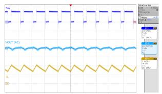
Figure 5-8. Steady State,  $V_{IN}$  = 9V,  $I_{OUT}$  = 1.2A
