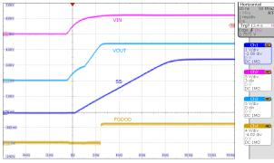
Figure 5-9. Start-Up,  $V_{IN} = 3.3V$ ,  $I_{OUT} = 0.6A$
