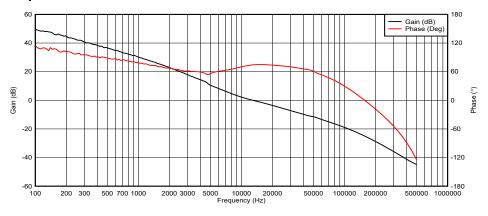
Figure 5-15. Control Loop Response,  $V_{IN} = 3.3V$ ,  $I_{OUT} = 0.6A$
