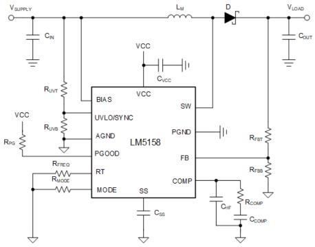
Figure 2-1. Application Circuit
