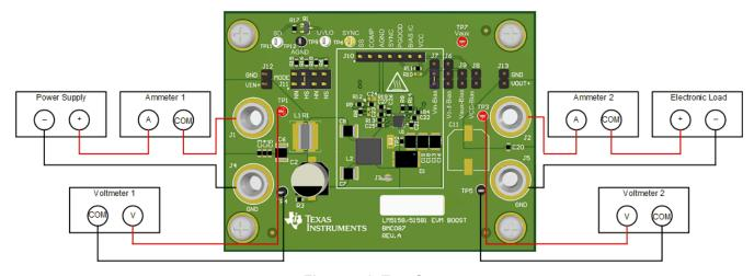
Figure 4-1. Test Setup
