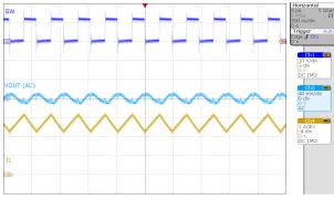
Figure 5-6. Steady State,  $V_{IN}$  = 3.3V,  $I_{OUT}$  = 0.6A
