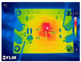
Figure 5-4. Thermal Image:  $V_{IN}$  = 3.3V,  $I_{OUT}$  = 0.6A,  $V_{BIAS}$  = 12V, No Forced Air Cooling
