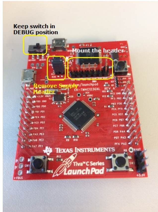
Figure 11. Preparing EK-TM4C123GXL as a Debug Probe
