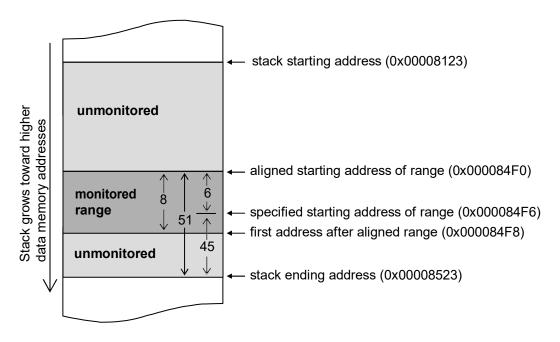
Figure 2. Watchpoint Range in Relation to the Stack in Memory (numerical values refer to specific example given in the text)
