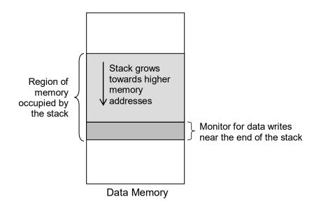
Figure 1. Stack Overflow Monitoring
