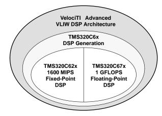
Figure 1. TMS320C6000 Generation of DSPs
