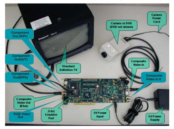
Figure 1. Hardware Setup
