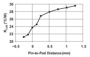
Figure 1-3.  $R_{\theta JA}$  vs Pin-to-Pad Distance
