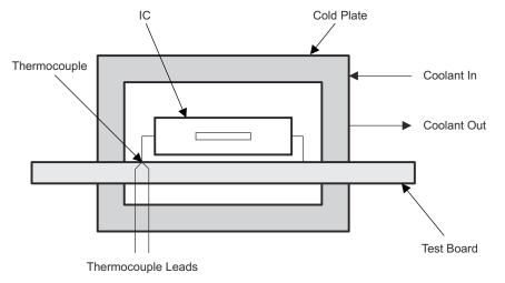
Figure 4-2.  $R_{\theta(JB)}$  Measurement Method
