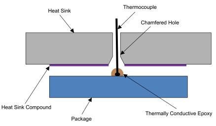
Figure 3-1. Installing a Heat Sink With Thermocouple
