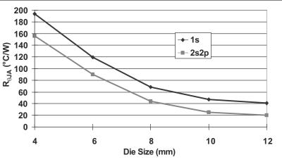
Figure 1-2. Die Size Impact on a CSP
